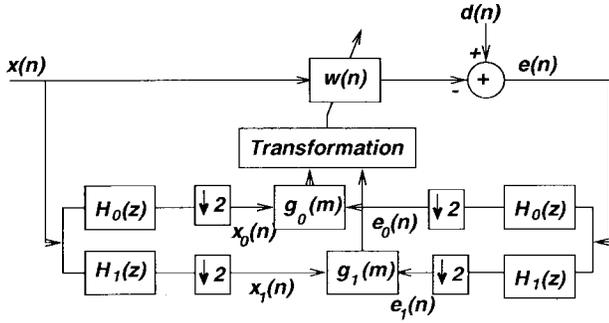
Fig. 1. Structure of the delayless subband adaptive filter.
