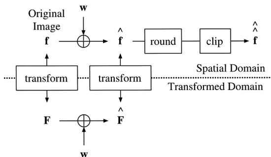
Fig. 1 Block diagram of data embedding.
