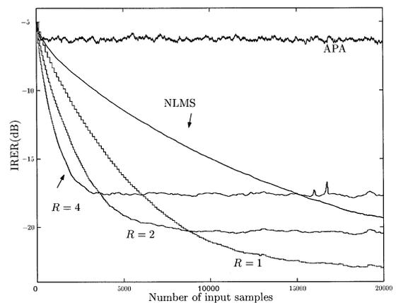
**Fig. 9** Results of simulation when the signal-to-noise ratio was  $-20$  dB. The length of adaptive filter and the unknown system were 151.
