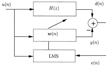
**Fig. 1** Configuration of the system identification considered in this paper.
