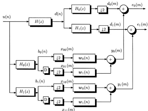
**Fig. 2** Configuration of the AFSAF when the number of channel is two.  $D$  shows a unit delay.
