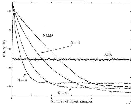
**Fig. 7** Results of simulation when the signal-to-noise ratio was  $-50$  dB.
