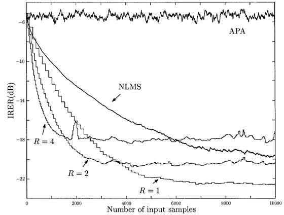
**Fig. 8** Results of simulation when the signal-to-noise ratio was  $-20$  dB. The length of adaptive filter and the unknown system were 61.
