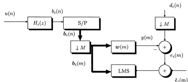
**Fig. 4** An equivalent structure of the  $i$ -th channel of AFSAF. S/P shows a serial to parallel converter. A bold line shows that the signal is a vector and a thin line shows a scalar.  $\tilde{e}_i(m)$  shows the sum of the error signals from other channels
