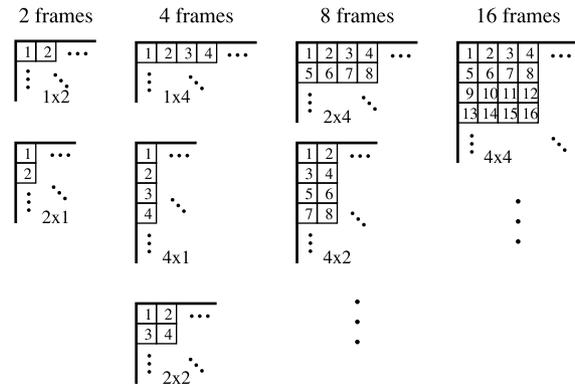
Fig. 3 Example of generating a large picture from 2, 4, 8, and 16 frames. Interleaving is performed for each pixel of each frame.
