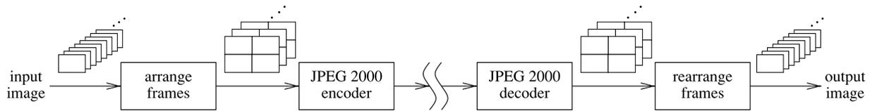
Fig. 1 Conventional method that generates a large picture as an input for the JPEG 2000 encoder.
