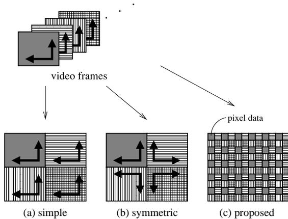
Fig. 2 Methods for generating a large picture from four frames.
