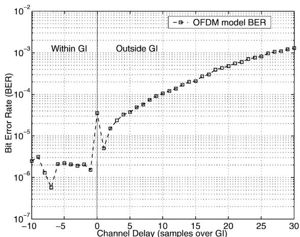
Fig. 6 Channel delay vs. BER in the simulated OFDM system.
