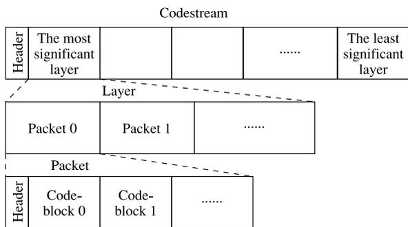
Fig. 1 Structure of a JPEG2000 codestream.
