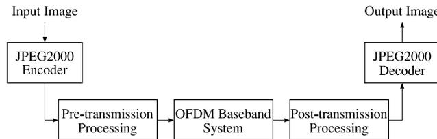
Fig. 3 Proposed method in JPEG2000-coded image transmission over OFDM system.
