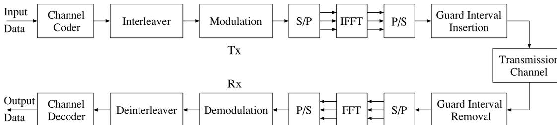
Fig. 2 OFDM baseband system architecture.
