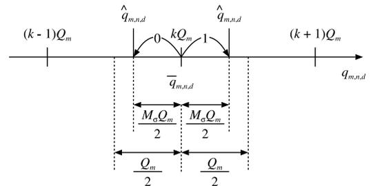
**Fig. 4** Chosen coefficient  $q_{m,n,d}$ , its rounded value  $\bar{q}_{m,n,d}$ , and watermarked coefficient  $\hat{q}_{m,n,d}$  in embedding binary watermark sequence  $\mathbf{w}_g$ .  $k$  is an integer. Embedding '0' and '1' result in  $\hat{q}_{m,n,d} = \bar{q}_{m,n,d} - M_\sigma Q_m / 2$  and  $\hat{q}_{m,n,d} = \bar{q}_{m,n,d} + M_\sigma Q_m / 2$ , respectively. Rounding both  $\hat{q}_{m,n,d}$ 's off results in  $\bar{q}_{m,n,d}$ .  $M_\sigma$  controls  $\max_l |\hat{w}_{g,l}|$ .
