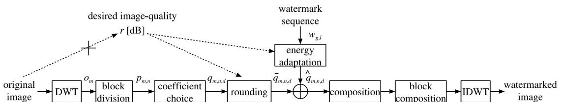
Fig. 3 Embedding diagram of the proposed IQGW method.
