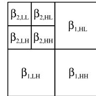
**Fig. 2** Subband  $\beta_{\lambda,\theta}$  in a two-dimensional DWT. (Decomposition level  $\Lambda = 2$ . Parameters  $\lambda$  and  $\theta$  represent the resolution level and the direction, where  $\theta \in \{\text{LL}, \text{LH}, \text{HL}, \text{HH}\}$ ).
