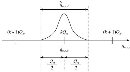
**Fig. 5** Chosen coefficient  $q_{m,n,d}$ , its rounded value  $\bar{q}_{m,n,d}$ , and watermarked coefficient  $\hat{q}_{m,n,d}$  in embedding spread spectrum-based watermark sequence  $w_g$ .  $k$  is an integer. Rounding  $\hat{q}_{m,n,d}$ 's off results in  $\bar{q}_{m,n,d}$ .
