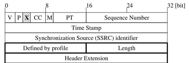
**Fig. 4** Structure of RTP header.
