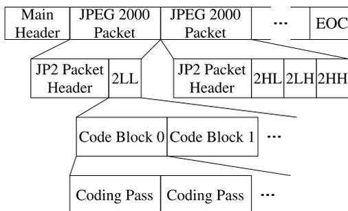
Fig. 3 Structure of code stream of JPEG 2000 coded image.
