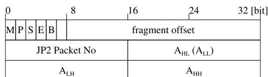
**Fig. 9** Structure of the extended part of RTP header for the packet containing JPEG 2000 packet headers.
