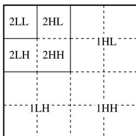
Fig. 1 Division into code blocks based on the wavelet transform.
