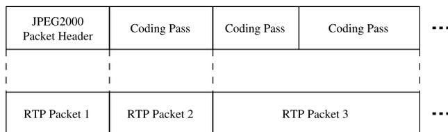
Fig. 6 Decomposition of JPEG 2000 code stream in RTP packets.
