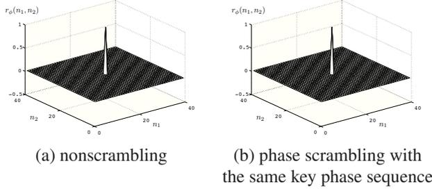
**Fig. 4.** Blind image matching. POC surfaces (a) and (b) are identical. The same accuracy is obtained from invisible images protected by phase scrambling.
