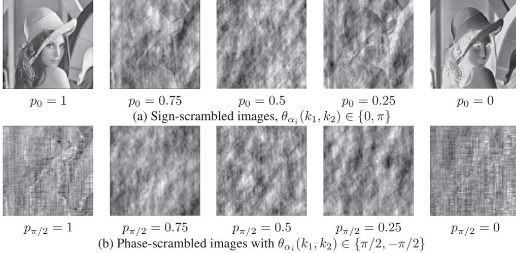
**Fig. 2.** Sign-scrambled images and phase-scrambled images. (a)  $p_0$  affects the effect of visual protection in sign-scrambled images. (b) Phase scrambling protects the contents of original image, regardless of  $p_{\pi/2}$ , except for the case in which  $p_{\pi/2} = 1$ .
