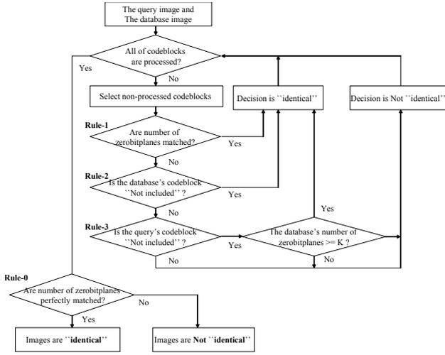
**Fig. 7.** Procedure of identification for encrypted JPEG 2000 images.
