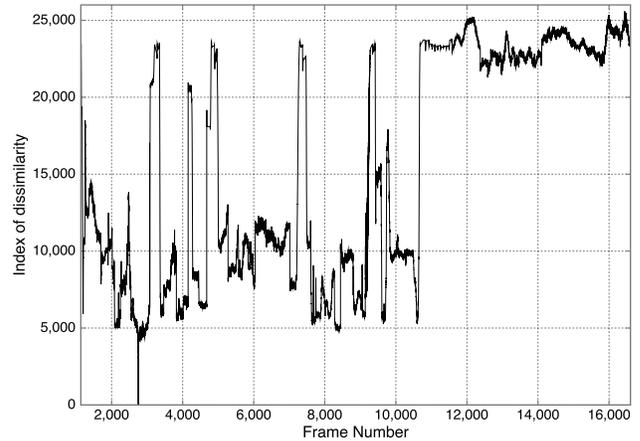
**Fig. 9.** Index of dissimilarity when 2750th frame was used as query image. The zero dissimilarity at 2750th frame shows that proposed method correctly identified database image matching query image.
