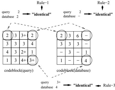
**Fig. 6.** Rules of codeblock identification("Not included" in query is transformed to  $K+$ )
