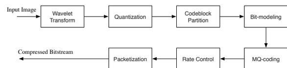
Fig. 1. Block diagram of JPEG 2000 encoder
