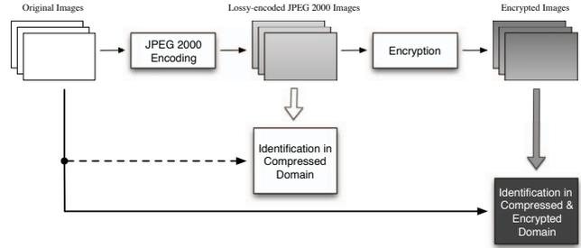
**Fig. 4.** Model of image identification: dashed line and solid line is equal to the conventional method and the proposed method, respectively.
