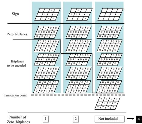
**Fig. 5.** Re-definition of number of zero-bit-planes: The third codeblock is re-defined as "4+", instead of "not included". It is because 4 zero-bit-planes actually exist. But if there were non-zero-bit-planes before truncation in the LSB direction, the number of bit-planes would be 4 or more.
