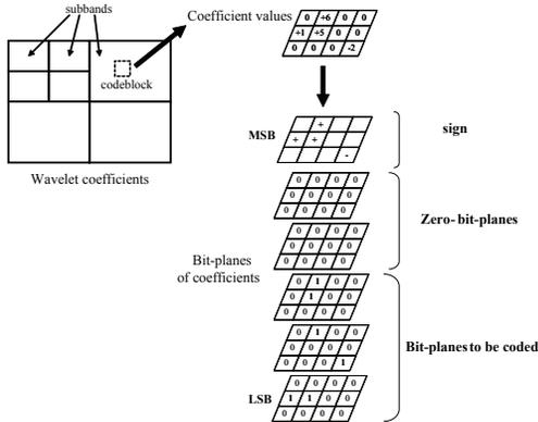
**Fig. 2.** Code Blocks and bit-planes: Zero-bit-plane is a special bit-plane in which samples are all zeros. Zero-bit-planes are arranged from MSB level to LSB level.
