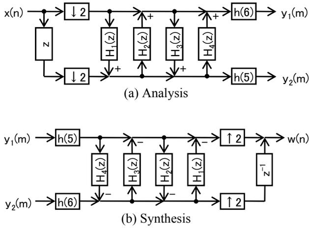
Fig.1 Implementation of DWT in the 'lifting' form.
