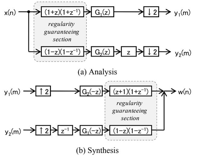
Fig.3 DWT in the proposed 'non-lifting' form (type A). It guarantees the regularity.
