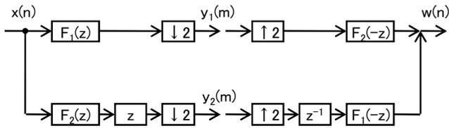
Fig.2 DWT in the 'filter bank' form.
