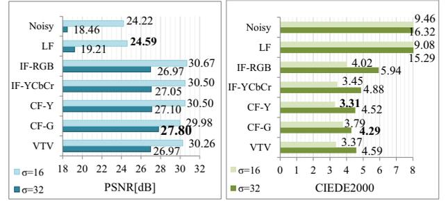
Figure 4: PSNR and CIEDE2000 comparison for the denoising of the *Parrots* color image with  $\sigma = 16, 32$ .
