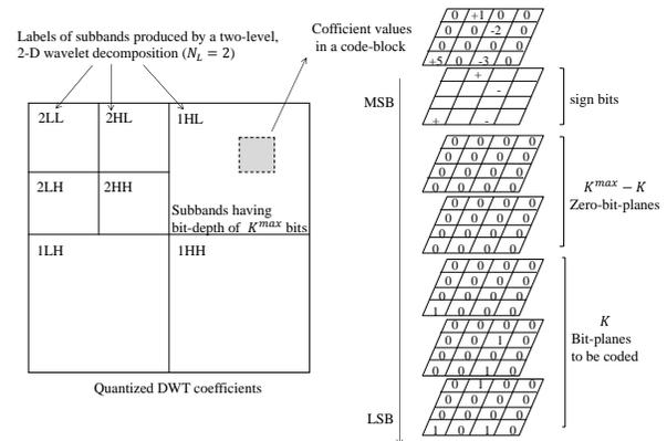
Fig. 2. Bit-plane decomposition and sign-magnitude representation of DWT coefficients in code-block. A zero-bit-plane is a special bit-plane in which the samples are all zeros. Zero-bit-planes are arranged from the MSB to the LSB level.
