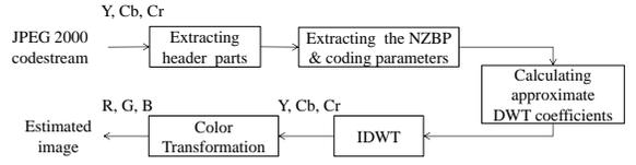
Fig. 4. Block diagram of the proposed estimation.
