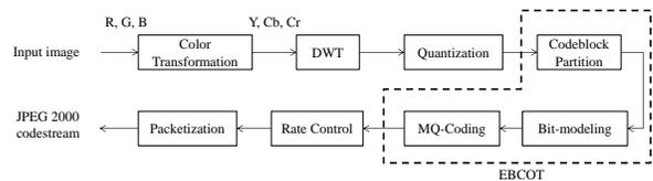
Fig. 1. Block diagram of JPEG 2000 encoder.
