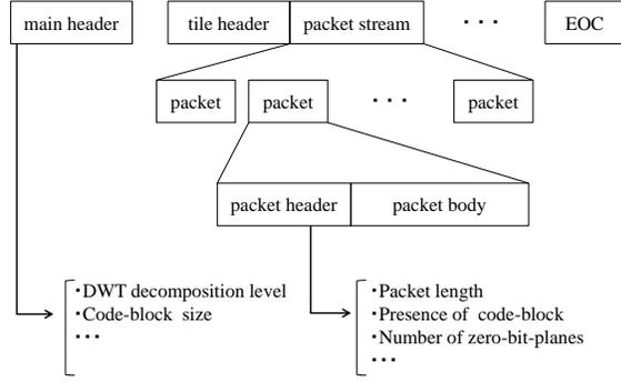
Fig. 3. Structure of JPEG 2000 codestreams.
