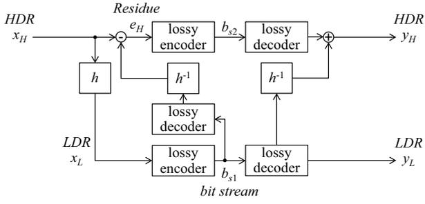
Fig. 1: A two layer backward compatible ‘lossy’ coding system. The encoder outputs two kinds of bit streams  $b_{s1}$  and  $b_{s2}$ . The decoder reconstructs an LDR image  $y_L$  from  $b_{s1}$ , and an HDR image  $y_H$  from  $b_{s1}$  and  $b_{s2}$ . Both of  $y_L$  and  $y_H$  contain quantization errors.
