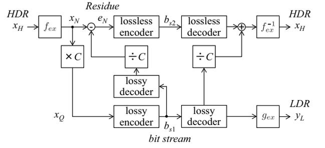
Fig. 3: The existing method in [14]. It reconstructs HDR image  $x_H$  without any loss. The reversible logarithmic mapping  $f_{ex}$  was introduced to reduce the range of HDR pixel values. The mapping  $g_{ex}$  is additionally introduced to compensate the effect of  $f_{ex}$ .
