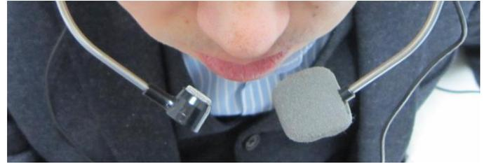
Fig. 4. Headset microphone with a pop filter (right) and that without any pop filter (left).
