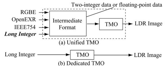
**Fig. 1** The scheme of a unified tone mapping operation.
