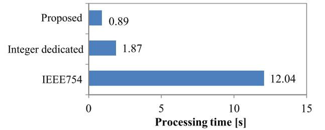
**Fig. 3** The processing time of the methods. This experiment applied tone mapping for HDR images with  $512 \times 768$  pixels in the integer format using each method.
