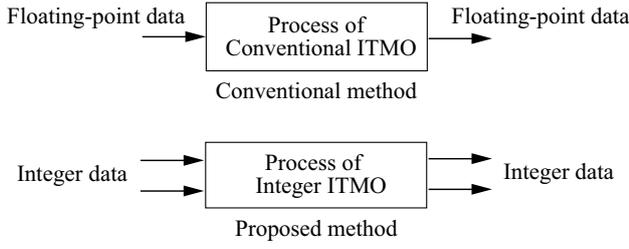
**Fig. 2.** The difference between the conventional method and the proposed integer ITMO.
