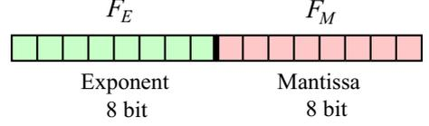
Fig. 1. The bit allocation of the proposed intermediate format.
