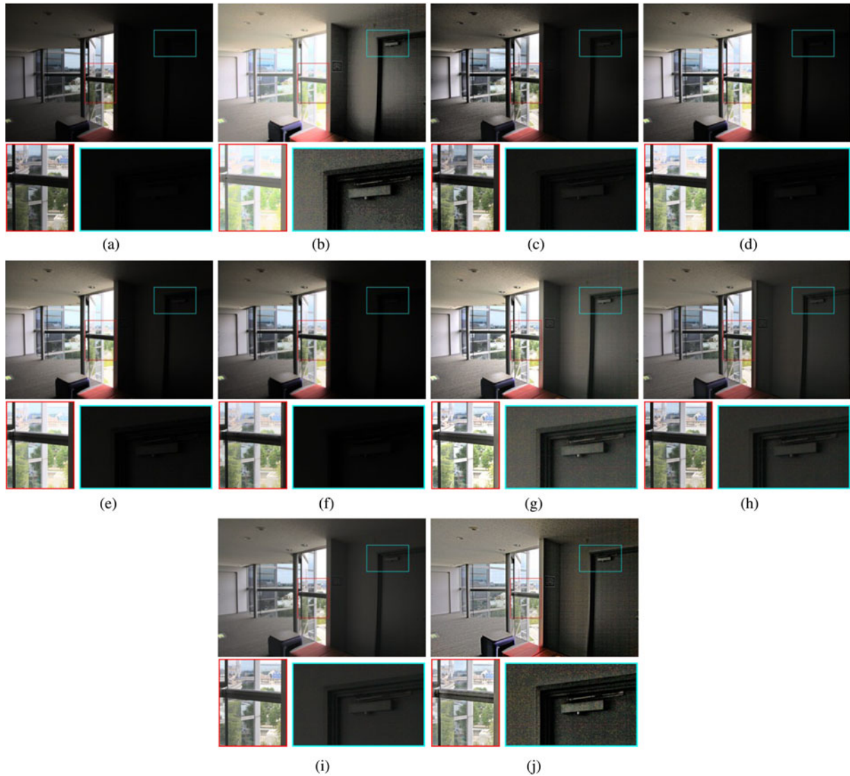
Fig. 7. Comparison of the proposed method with image-enhancement methods (Window). Zoom-ins of boxed regions are shown in bottom of each image. The proposed method can produce clear images without under- or over-enhancement. (a) Input image x ( -1EV ). Entropy: 3.811. Naturalness: 0.0058. (b) HE. Entropy: 5.636. Naturalness: 0.6317. (c) CLAHE [1]. Entropy: 5.040. Naturalness: 0.0945. (d) AGCWD [2]. Entropy: 5.158. Naturalness: 0.1544. (e) CACHE [3]. Entropy: 5.350. Naturalness: 0.1810. (f) LLIE [6]. Entropy: 4.730. Naturalness: 0.0608. (g) LIME [4]. Entropy: 7.094. Naturalness: 0.9284. (h) SRIE [5]. Entropy: 5.950. Naturalness: 0.2548. (i) BIMEF [21]. Entropy: 5.967. Naturalness: 0.2181. (j) Proposed. Entropy: 6.652. Naturalness: 0.7761.
