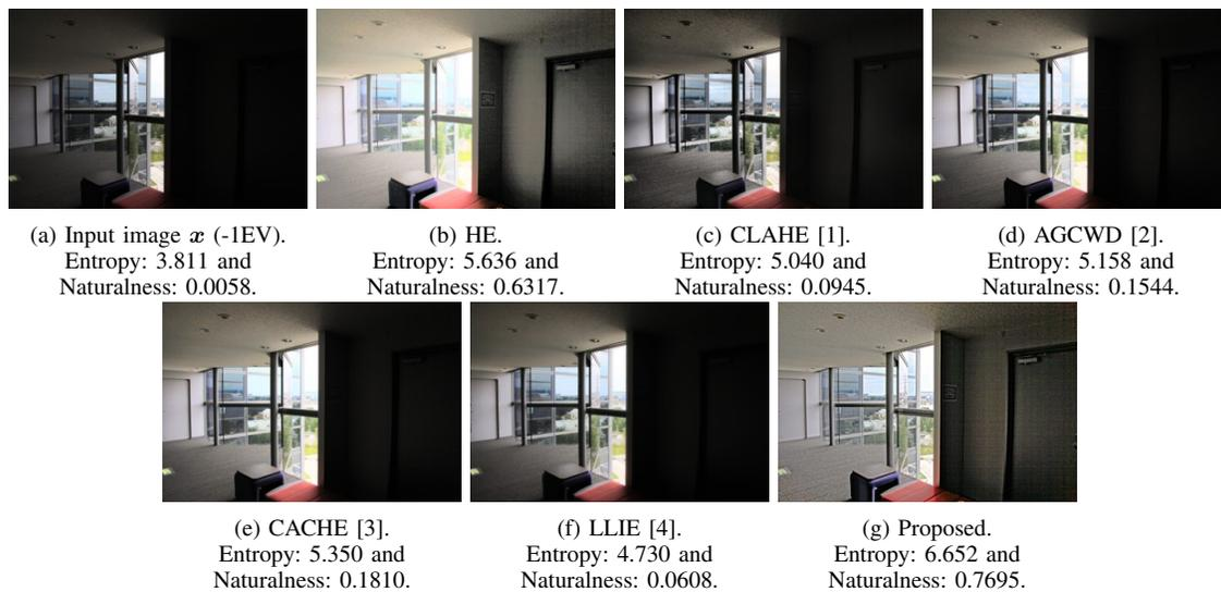
Fig. 5: Comparison of the proposed method with image enhancement methods (Window). The proposed method can produce clear images without under or over enhancement.
